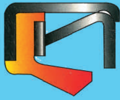
VA Outer metal case with reinforcing cap, sealing lip
